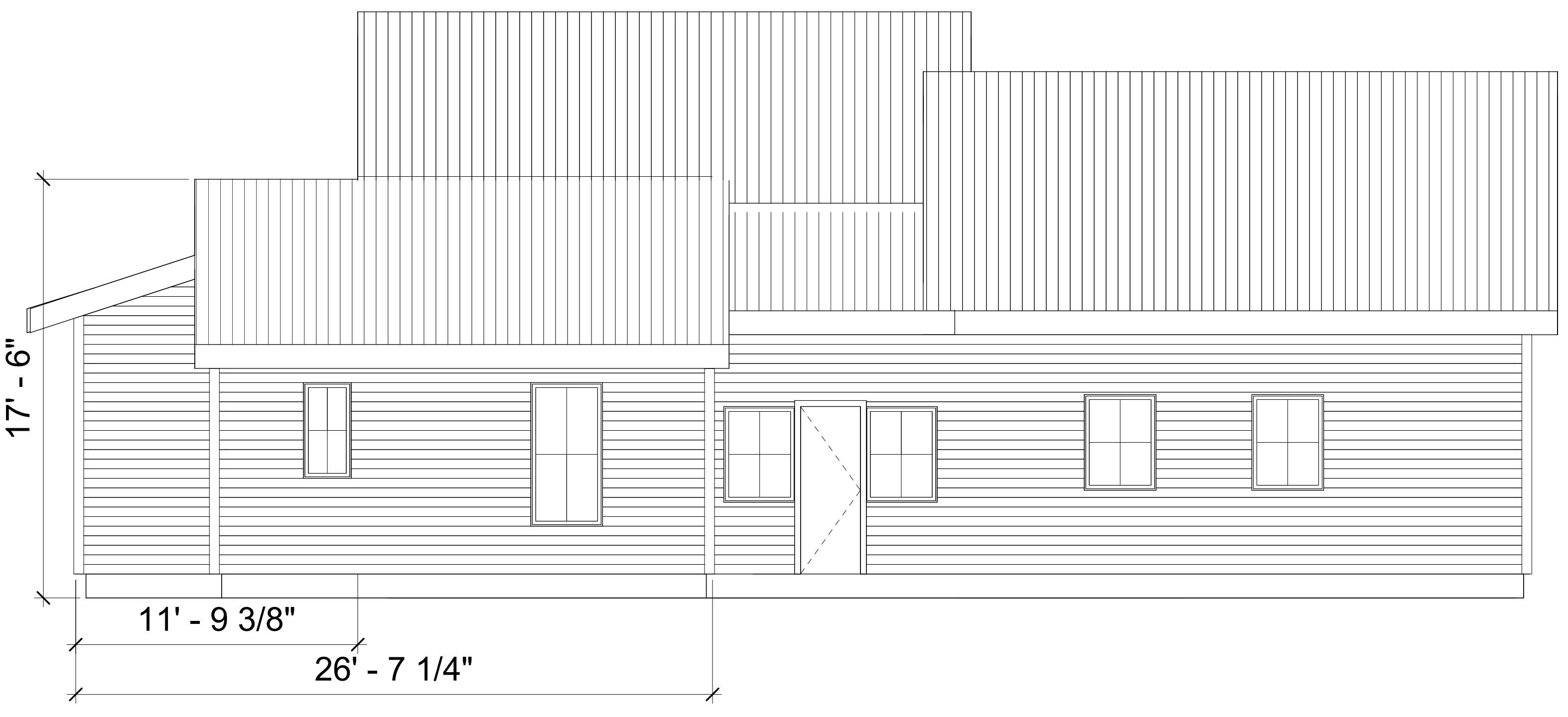
3 North Elevation - Backside 1/4" = 1'-0"
