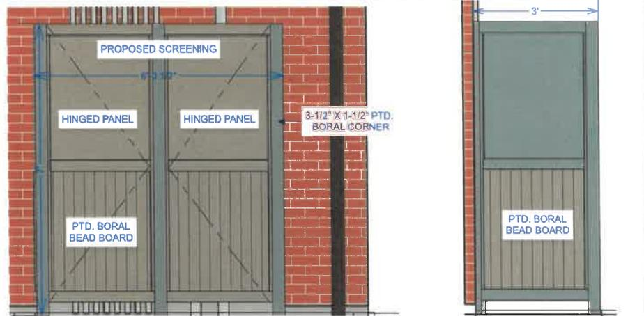
ELEVATIONS - METER ENCLOSURE SCALE 1/2" = 1'-0"
